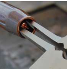
Spatter removal from inside the nozzle
